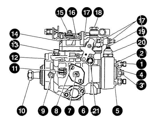
10 = Hexagon nut 60..70 Nm Thread M12 / taper 17 mm Part no. 2 915 011 011
